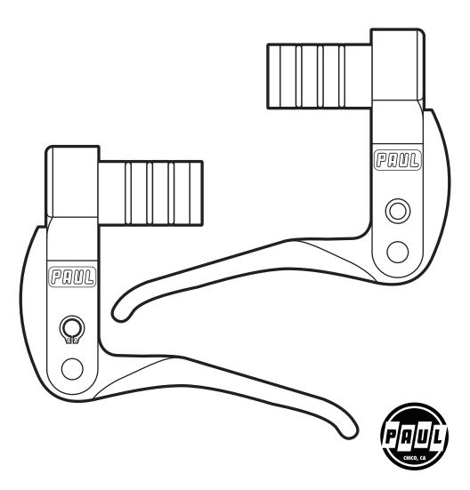
Congratulations on this purchase, we really appreciate it! These levers plug into the end of compatible handlebars. They fit bores from 19mm to 22mm. They are compatible with probably every cable bicycle brake ever made. The housing/cable will run alongside the bottom of the bars and should be covered in handlebar tape. The levers are ambidextrous.
